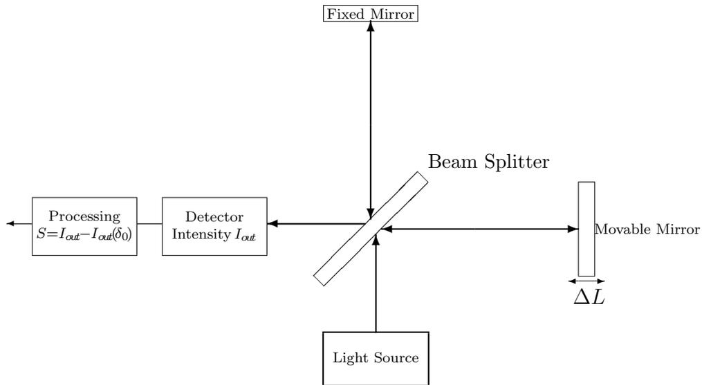
The Figure shows a Michelson interferometer in which two coherent light waves, derived from the same monochromatic source, are combined into one wave of intensity  $I_{out}$ . This intensity is measured and processed into a signal  $S$  that is sensitive to small displacements  $\Delta L$  of a movable mirror relative to some reference position. You will determine the optimum reference configuration according to two different criteria, and explain any difference.
